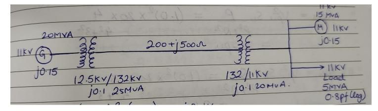
Problem statement – In the previous question, if the motor is a synchronous machine drawing 15 MVA at 0.9 power factor (leading) and terminal voltage 1.1 pu. Find the generator bus voltage. (Answer - 1.3238; 28.71 degree)
